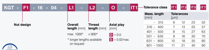
Nominal diameter 16.0 mm | Lead 5.0 mm Max. speed 4200 rpm | Ball diameter 3.50 mm
