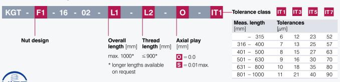
Nominal diameter 16.0 mm | Lead 2.5 mm Max. speed 3500 rpm | Ball diameter 1.60 mm
