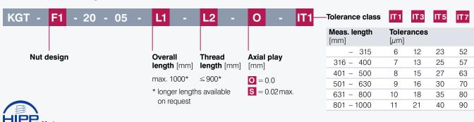
Nominal diameter 20.0 mm | Lead 5.0 mm Max. speed 4000 rpm | Ball diameter 3.50 mm | Pre-loaded double nut
