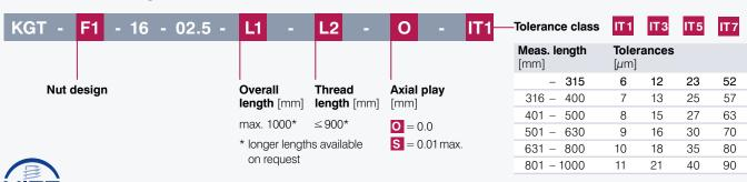
Moving Precision Nominal diameter 16.0 mm | Lead 4.0 mm Max. speed 4000 rpm | Ball diameter 2.50 mm
