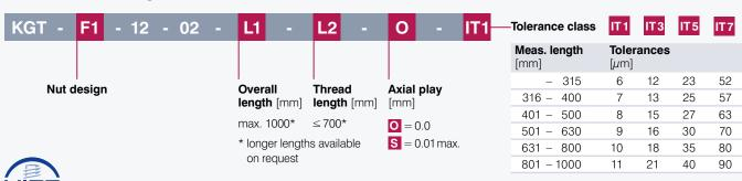
Nominal diameter 12.0 mm | Lead 2.5 mm Max. speed 3800 rpm | Ball diameter 1.60 mm
