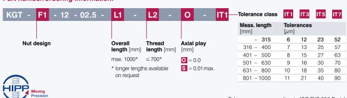
Nominal diameter 12.0 mm | Lead 3.0 mm Max. speed 4000 rpm | Ball diameter 1.60 mm
