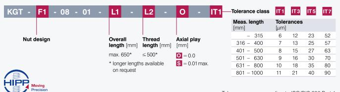
Nominal diameter 8.0 mm | Lead 2.0 mm Max. speed 4500 rpm | Ball diameter 1.60 mm
