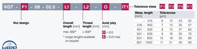
Nominal diameter 8.0 mm | Lead 3.0 mm Max. speed 4500 rpm | Ball diameter 1.60 mm
