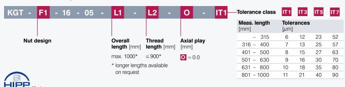
Nominal diameter 16.0 mm | Lead 10.0 mm Max. speed 4200 rpm | Ball diameter 3.50 mm
