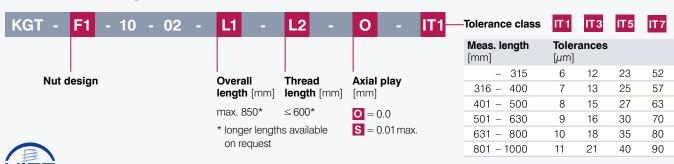
Nominal diameter 10.0 mm | Lead 2.5 mm Max. speed 4000 rpm | Ball diameter 1.60 mm
