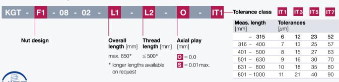
Moving Precision Nominal diameter 8.0 mm | Lead 2.5 mm Max. speed 4500 rpm | Ball diameter 1.60 mm
