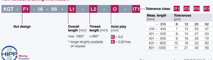
Nominal diameter 16.0 mm | Lead 5.0 mm Max. speed 4200 rpm | Ball diameter 3.50 mm | Pre-loaded double nut
