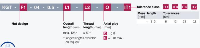
Nominal diameter 4.0 mm | Lead 1.0 mm Max. speed 4500 rpm | Ball diameter 0.80 mm
